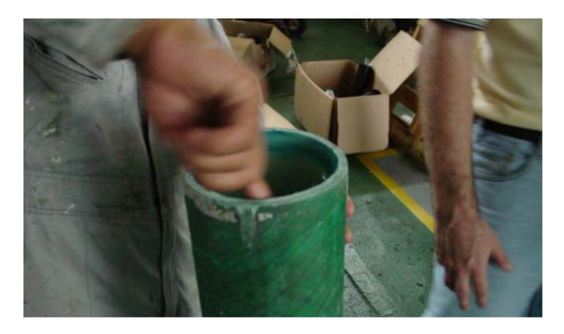
Carefully inspect the inside surface of the liner to insure that it is smooth and free of imperfections.
