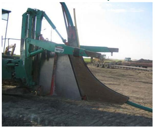
Shoe radius must be equal to or greater than the minimum bending radius of the FS LP being installed.
