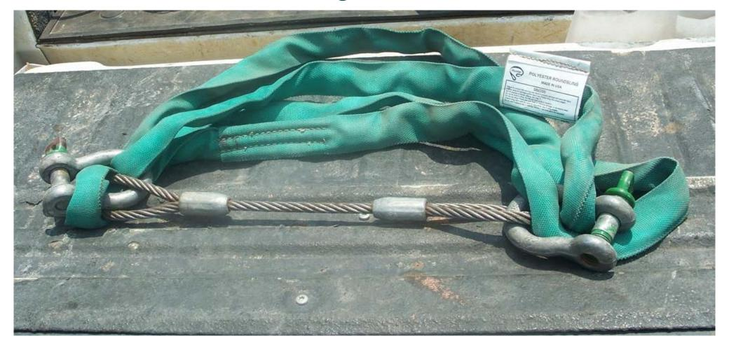
Shear Loop with Safety Sling attached
