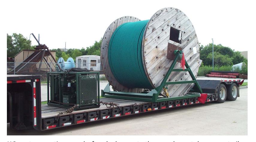
When transporting spools for deployment, the spool must be on a trailer, mounted in a suitable spooling frame. The trailer should be as close to the ground as practical. Be aware of overhead obstructions. The flanges of the spool should be in contact with the deck of the trailer during transportation and then raised after arrival on location.
