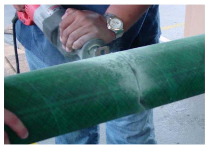
Fiberspar LinePipe is cut with a Sawzall using bi-metallic blades with 8/12 teeth per inch.
