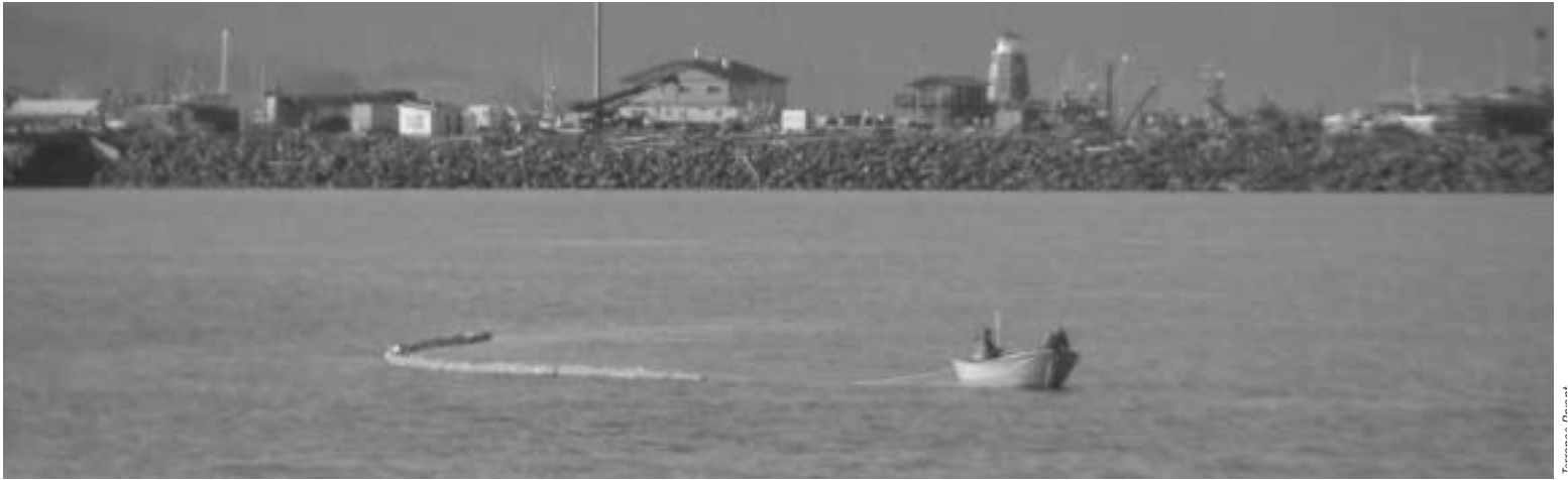
A skiff pulls ocean boom into place during the VOSS (Vessels of Opportunity) oil spill drill in Kachemak Bay. The exercise engages local vessels during the initial response to an oil spill.
