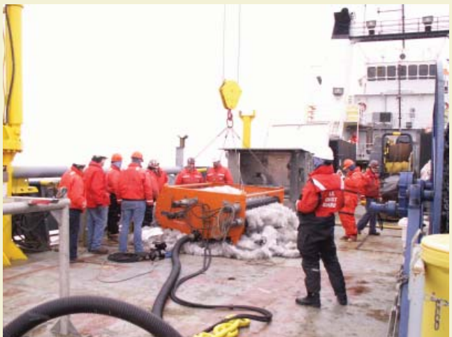
Observers study the V.A.B. oil skimmer on the deck of the Seabulk Nevada.
