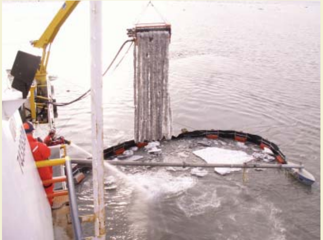
A CISPRI spill technician washes ice with a fire monitor, as the V.A.B oil skimmer simulates pulling oil from the water
