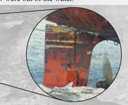
The Offshore Supply Vessel Monarch was pushed by ice into the offshore platform Granite Point, resulting in the sinking of the vessel. The tug Vigilant arrived too late.
