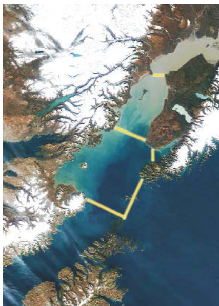
Location of transect where temperature and salinity profiles are providing information about density-driven currents in Cook Inlet and at its boundaries.
