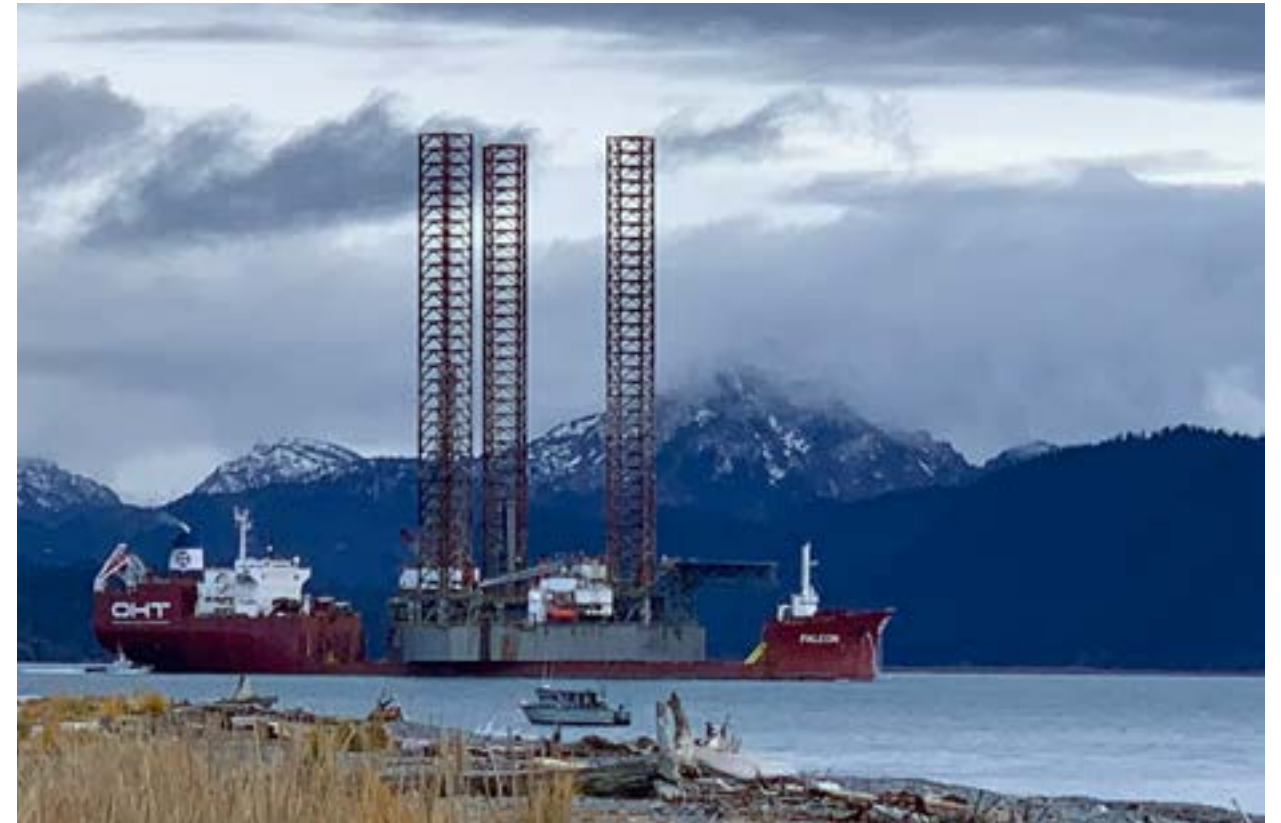
The jack-up rig Randolph Yost being being loaded onto the heavy lift vessel FALCON in Kachemak Bay, October 2021 for transport out of
