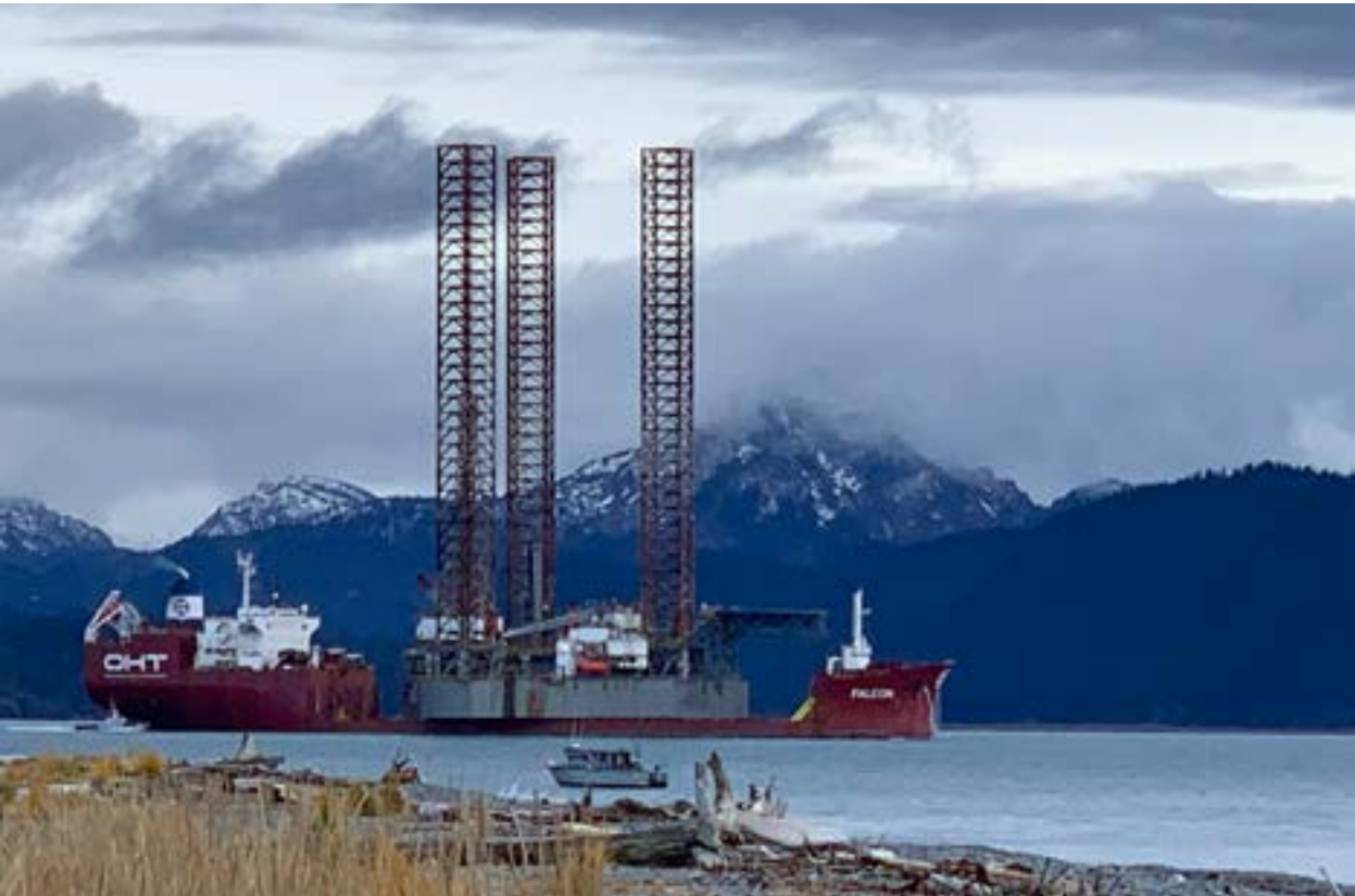
The jack-up rig Randolph Yost being being loaded onto the heavy lift vessel FALCON in Kachemak Bay, October 2021 for transport out of
