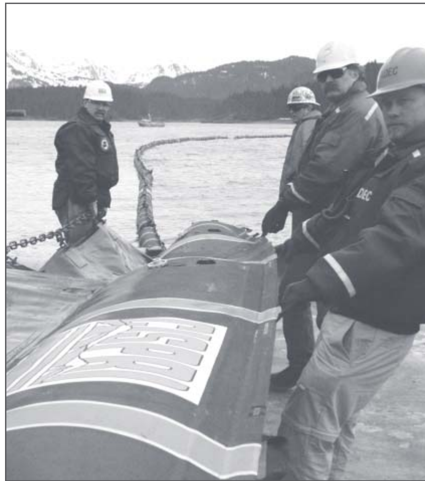
Responders deploy ocean boom from the CISPRI vessel Seabulk Montana during a recent VOSS drill in Jakalof Bay near Seldovia.
