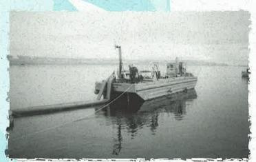
The 650-barrel oil spill responder barge and boom is deployed during a nearshore training exercise
