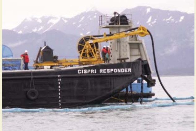
The barge CISPRI Responder, deploys a Transrec weir skimmer to oil recovery.
