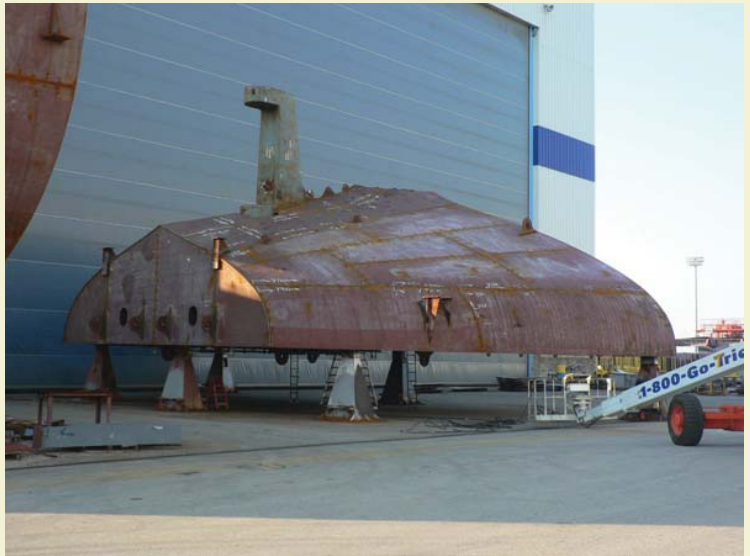
Overseas Martinez, a U.S. Flag Handysize Product Carrier, under construction at Aker Philadelphia Shipyard
